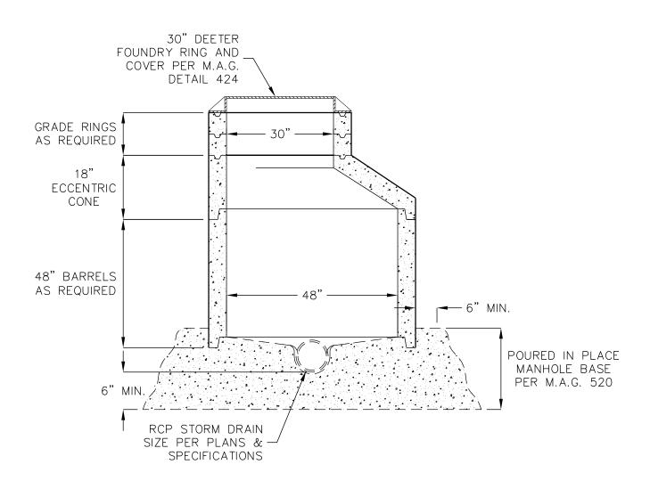
FOR COMPLETE DESIGN AND PRODUCT INFORMATION CONTACT JENSEN PRECAST. MANHOLE COMPONENTS CONFORM TO ASTM C-478 AND AASHTO M199.
