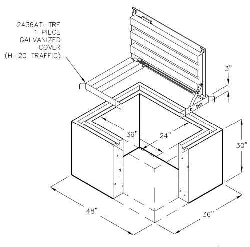
KNOCKOUTS, OPENINGS, HARDWARE, ETC. PER SOUTHWEST GAS SPECIFICATIONS.
