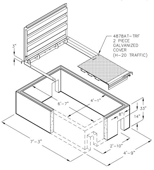
KNOCKOUTS, OPENINGS, HARDWARE, ETC. PER SOUTHWEST GAS SPECIFICATIONS.
